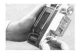
3. Wind up the shutter winding knob (5) as far as it will go in a clockwise direction, until a hard stop is felt. (A slight resistance may mean that the shutter is not fully wound, so that it is necessary to turn fully until the stop is reached.)
