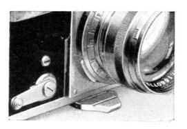
when the delayed-action mechanism is fully wound the shutter time may be set or the shutter wound up, but this can only be done with the delayed-action device either fully wound or else fully run down. In order to preserve the spring tension of the delayed-action mechanism, never leave it fully wound for any length of time.
