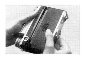
2. Draw the camera back slightly downwards, and then lift it away from the body of the instrument.
