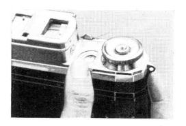
9. Give a half-turn to the locking keys on the under side of the camera to lock the back in place, and fold them flat once more.
