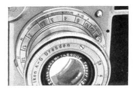
may be altered by turning the lens aperture ring to adjust it correctly.
