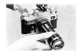
should be turned. When this is done, the focussing wheel (8) on the camera should also revolve.
