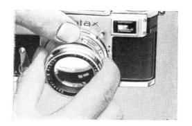
spring (18) so that the projection on the lens barrel, marked with a red dot, slides out of the spring catch holding it. A slight turn of the lens in a clockwise direction releases it, and it may then be carefully drawn out of the helical focussing mount.
