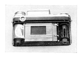
4. Place the Contax spool with its hollow end on the claw (21) of the left-hand spool chamber, and break the gumstrip that holds down the end of the paper leader.
