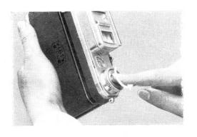
11. Press the shutter release button (6) lying in the centre of the shutter winding knob (this will work the shutter), and—holding it down—turn it in an anti-clockwise direction until a stop is felt. In this position the shutter button will stay permanently in the lower level.
