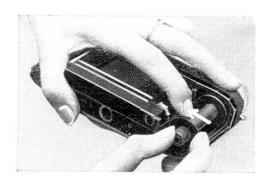
5. Pulling the leaf spring (25) towards the film sprocket with the left forefinger, take out the empty spool in the right-hand spool chamber.
