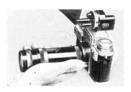
The removal of the lenses fitting the outer bayonet follows the procedure of inserting them. The side catch must first be lifted with the thumb, and then the lens is turned through 90° to the right, in which position it may be removed from the camera. The long-focus lenses are also coupled to the distance meter for focussing, and in order to make sure that the mechanism is working correctly, the focusing ring on the lens
