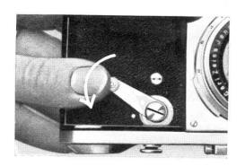
is first wound up in the normal way, and then the delayed-action mechanism is wound by pulling the lever (2) to the left (anticlockwise) as far as it will go.
