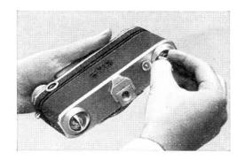
1. Open the camera by raising the two locking keys (19) on the camera base and giving them half a turn. In the open position the keys cannot be folded down against the camera body.
