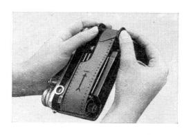
6. Now thread the end of the paper leader strip on the full spool into the wide slit of the empty spool, and when about 1 inch projects through on the far side, bend sharply backwards so that the black inner side of the paper faces outwards. Then replace the empty spool in the right-hand chamber with the claw (24) engaging in its hollow end.
