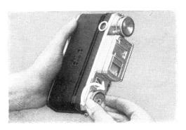
12. Wind up the shutter winding knob nine times, until the picture counter shows the number "36". If the rewinding knob (14) does not rotate during this operation, there is something wrong inside the camera, and the back must be removed to find out the cause of the trouble.
